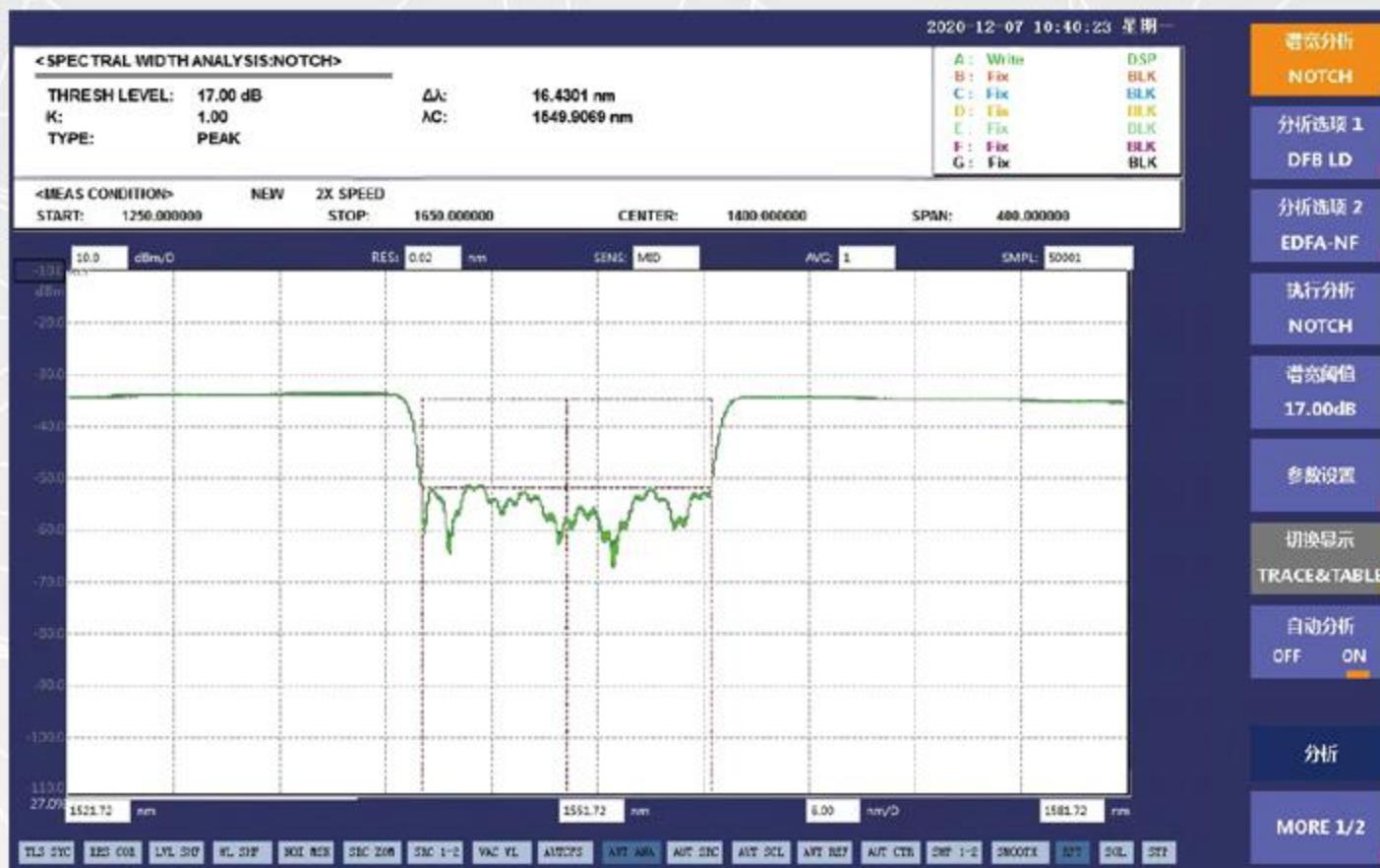
The AE8600A can measure the passband bandwidth or stopband bandwidth from the measured waveform of the V-characteristic or U-characteristic filter through notch bandwidth measurement.
