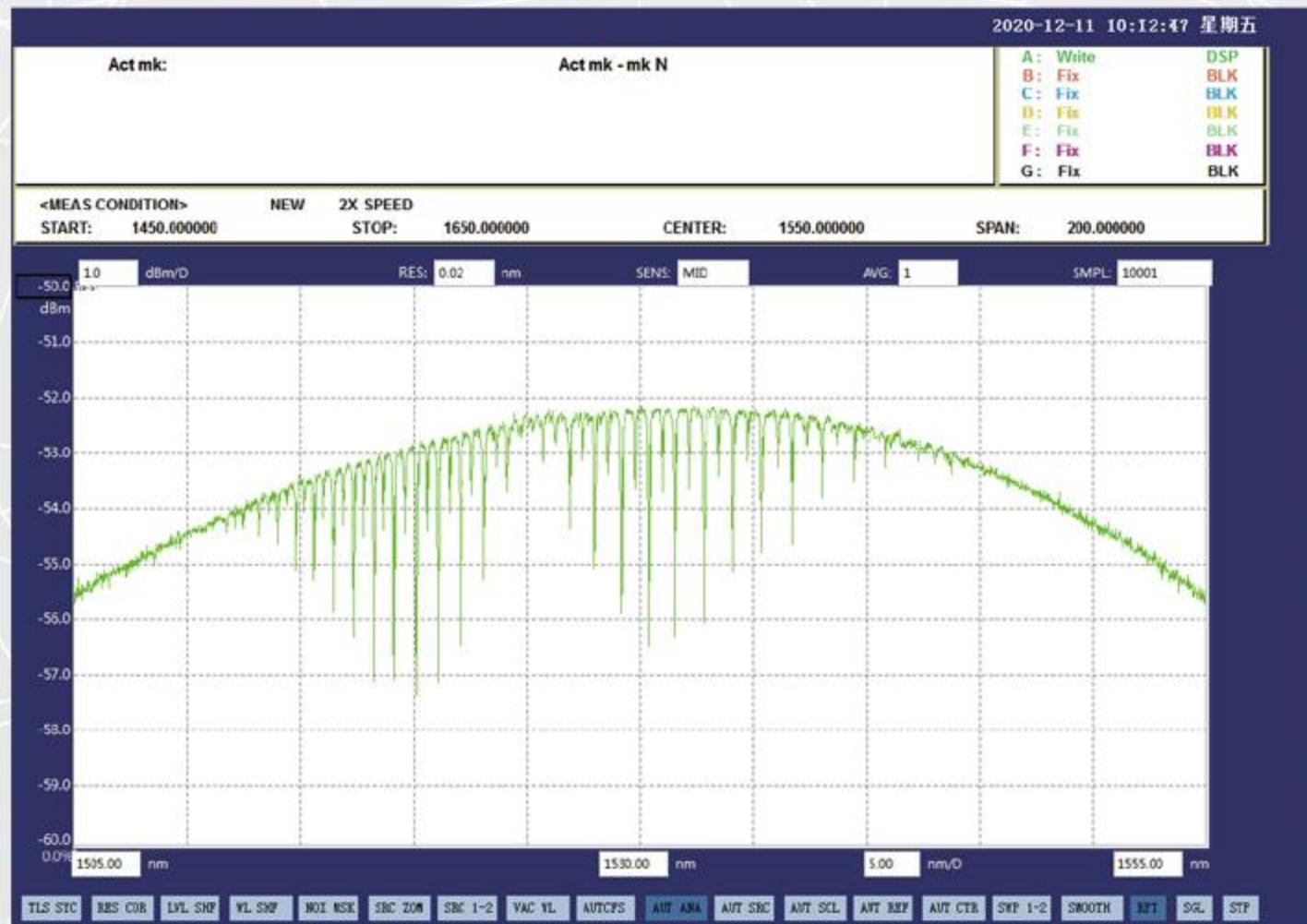
When used with broadband light sources such as supercontinuum (SC) or superluminescent diode (SLD), the AE8600A can display the optical absorption spectrum of the measured gas mixture.
