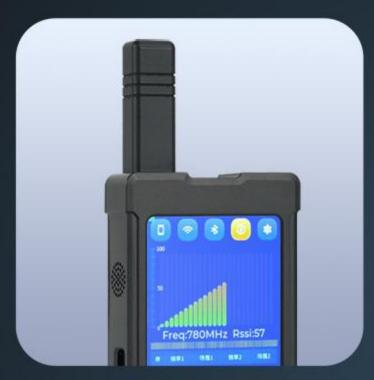
A separate 2.4GHz band detector supports 2.4GHz wireless camera device detection
