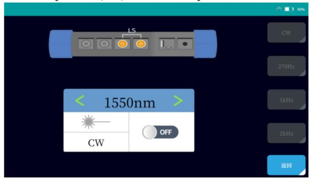
Step 1: Connect the LS interface (consistent with the QTDR interface);
