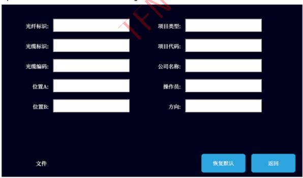
Save settings are used to set the SOR file saving content such as fiber optic identification, optical cable identification, optical cable coding, location and project type, project code, company name, operator, direction, etc.
