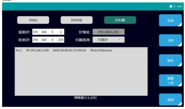
Connect to Ethernet LAN2, enter the starting scanning IP and ending scanning IP in the same IP section, and scan the IP used in this IP section.
