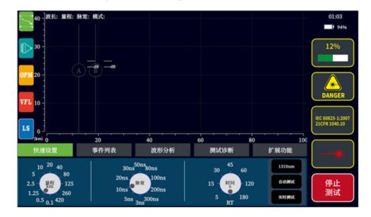
Note: Test parameters can be modified in real time during the test process (except for automatic test and multi-wavelength real-time test). Do not look directly at the output port.
