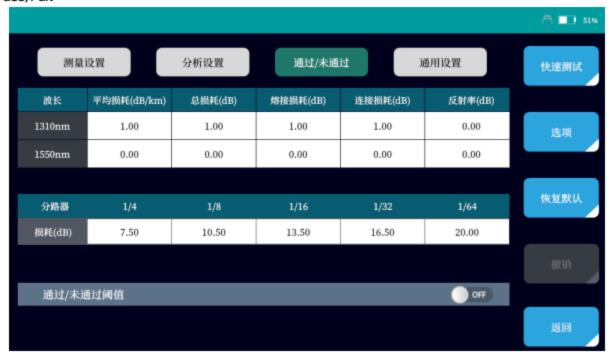
Pass/Fail is used to set Pass/Fail function parameters. It can set the average loss of different wavelengths, total link loss, splicing loss, connection loss, reflectivity and splitter loss judgment thresholds. If the set threshold is exceeded, an event will occur. mark in the list.
