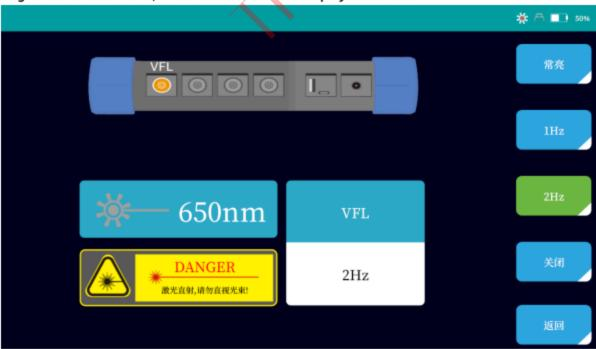
The red light function supports background operation and can remain on after exiting the operation interface.
