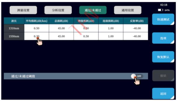
Pass/Fail is used to set Pass/Fail function parameters. The average loss of different wavelengths, total link loss, splice loss, connection loss and reflectivity judgment thresholds can be set. If the set threshold is exceeded, it will be marked in the event list.
