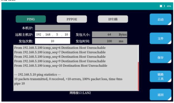
Connect to Ethernet LAN2, enter the remote host IP in the PING test, and click Start. Determine whether the Ethernet physical link is connected successfully. The test results can be saved as a txt format file.
