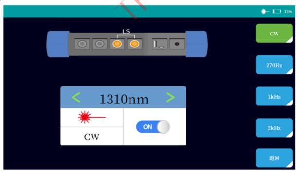
Switching the wavelength of the light source can be operated by clicking the "option key" in the picture above.
