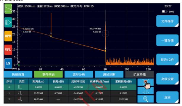
After the OTDR test completes the analysis, it automatically jumps to the curve operation interface. Click the zoom icon to zoom in on the event list.
