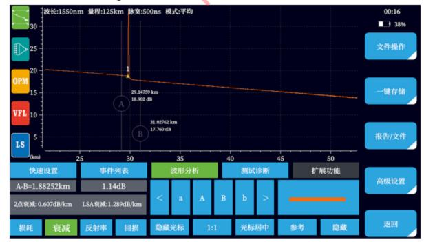
The 2-point method calculates the A-B cursor area attenuation in real time, and the LSA method calculates the A-B area attenuation in real time.
