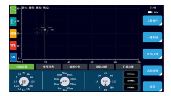
The setting interface is the first interface of the OTDR function: select the test range, pulse width, time, wavelength, and mode in sequence. Different ranges correspond to different optional pulse widths. RT is the real-time test mode, and the test time is selected as the average mode.
