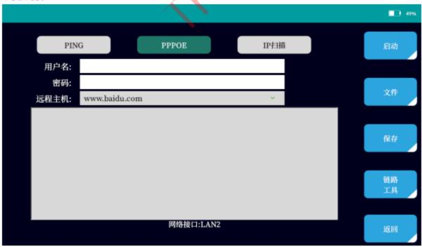
Connect to Ethernet LAN2, enter the user name and password in PPPOE, select the remote host, click Start, and determine whether the network can dial-up Internet access and whether network communication is normal.
