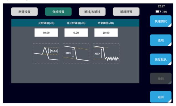
Set the reflection threshold, non-reflection threshold and end threshold required for event analysis.
