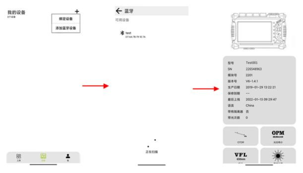
Step 3: The Bluetooth APP can control the light source function, optical power meter function (OPM) and red light function (VFL);
