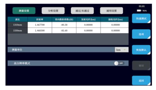
Set the refractive index, backs-cattering coefficient, transmitting fiber, receiving fiber, and measurement unit;
