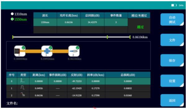
After the test is completed, the test results are displayed in two ways: event map and list. Click the corresponding wavelength to view the event list of each wavelength.
