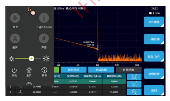
The quick operation interface controls the Bluetooth switch, Type-C USB (data transmission) switch, red light switch, quick screenshot, sound master switch, and brightness adjustment. It can also perform quick operations of shutting down and returning to the home page.
